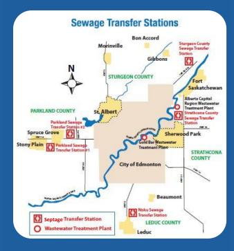
Wastewater discharged at the Hauled Waste Septage Receiving Stations is conveyed through a wastewater transmission network to either the ACRWC Wastewater Treatment Plant or to EPCOR's Gold Bar Wastewater Treatment Plant. There the wastewater is treated before it is discharged into the North Saskatchewan River.
